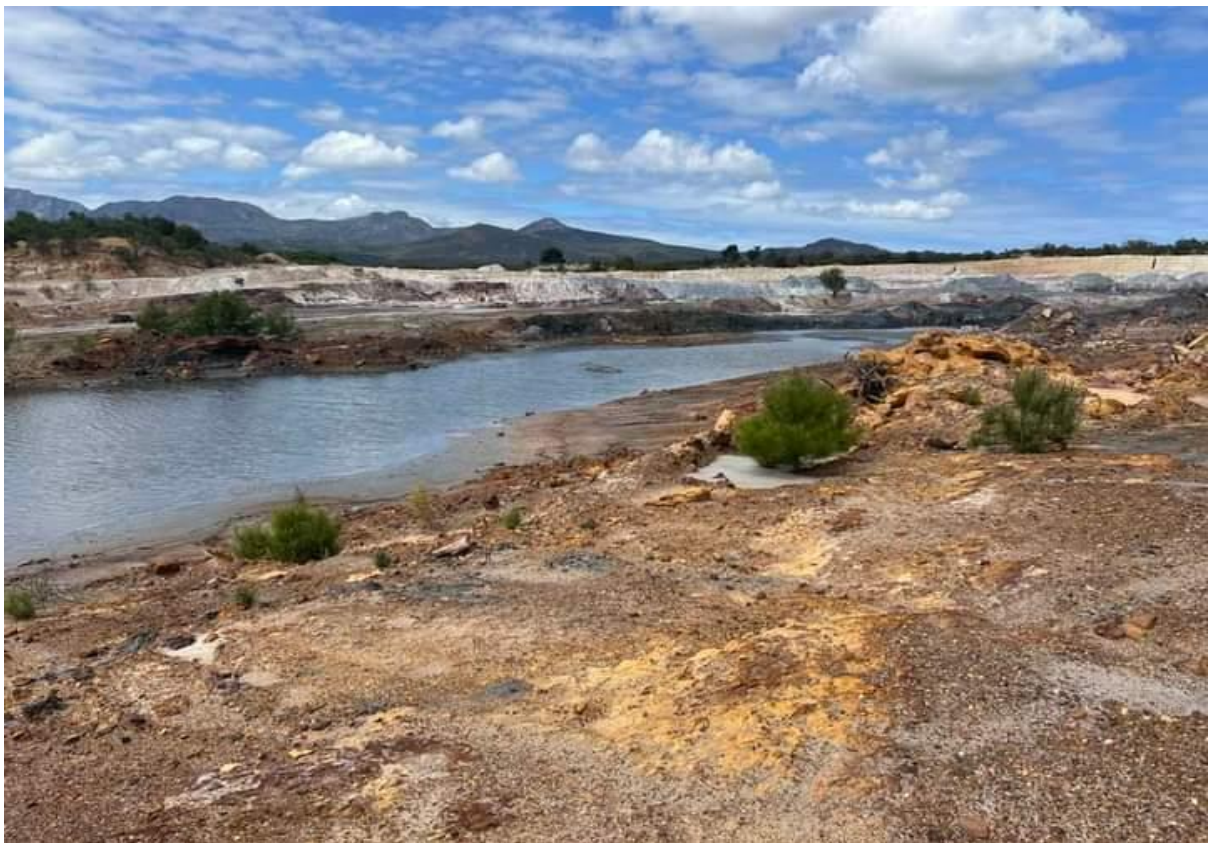
Botrivier Bricks Quarry - Bokkeveld shales and sediments used for Brick-making alongside the R43 between Hermanus and Bot River
